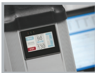
PLC controls with touch screen interface
